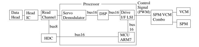
Notes: DSP controls actuator servo system. MCU controls spindle servo system.
